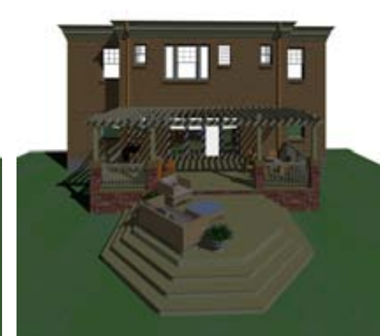
Modified 4 bay door (double hinged) Existing window removed and bricked in Composite (white) pergola, rail Stone siding Wood flooring
